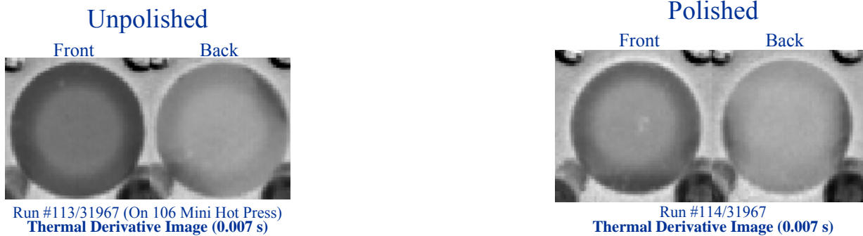
Figure 7. Results from pulsed thermography for the less polished pair of joined substrates (left) and for the more polished pair (right).
