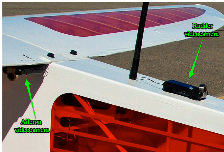
Figure 9: Videcameras used to record the control surface “failures”
