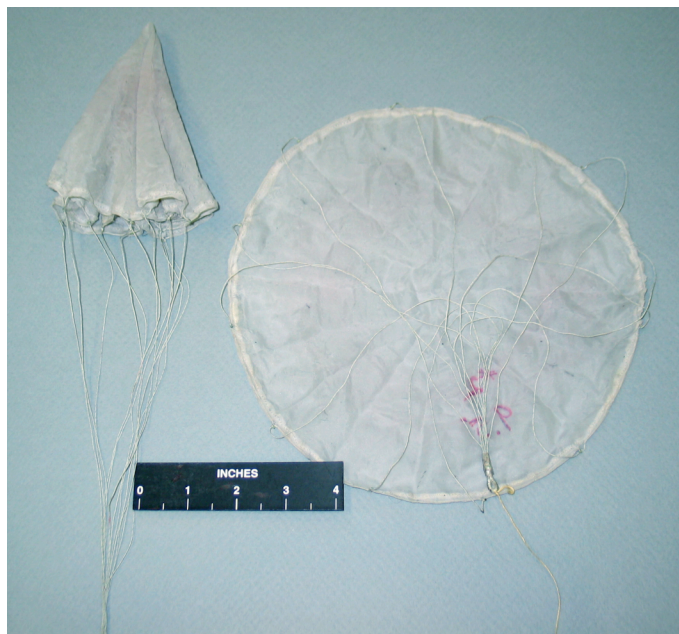
Figure 3. 9.5-inch flat circular parachutes used in drogue parachute tests in 20-Foot Vertical Spin Tunnel.
