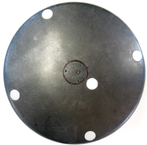
Figure 6. Retro-reflective targets affixed to model heat shield for tracking with optical data acquisition system.
