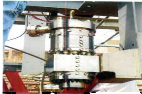
Figure 7. Full-scale workhorse gas generator in test stand at NASA MSFC
