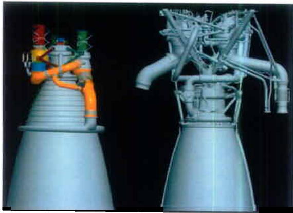
Figure 3. The J-2X engine shown in size comparison with the RS-68 booster engine
