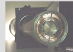
MSFC x-ray module with 12 nested mirrors
