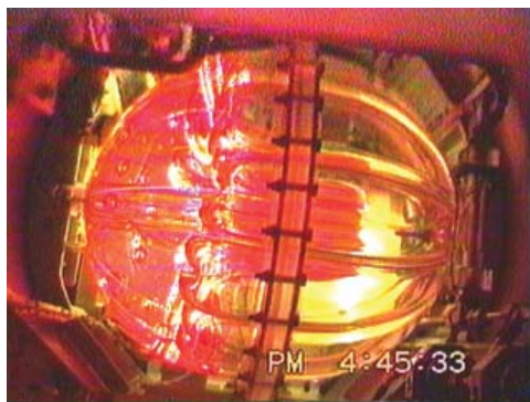
Figure 2.—Vented Tank Resupply Experiment during inflow, exhibiting center post fluid collection phenomena; predicted but unseen until VTRE flight.
