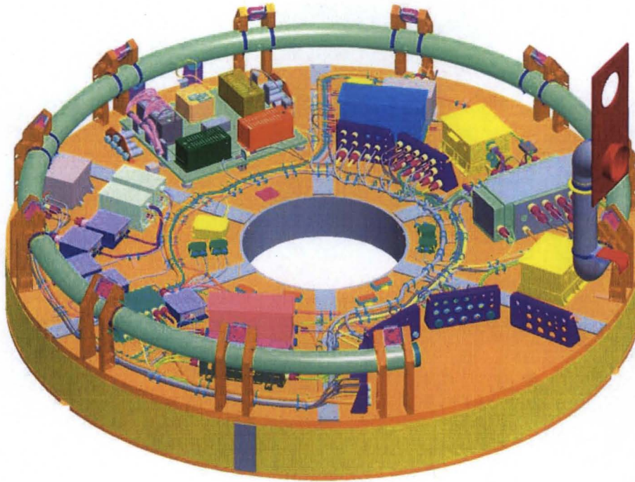
Figure 11. First Stage Avionics Module (FSAM) is provided by LMSS and located in the first stage fifth segment.
