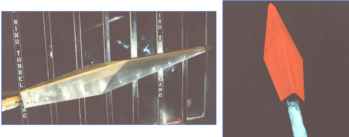
Fig. 5. Photographs of the faceted missile model installed in the test sections of NASA Langley Research Center wind tunnels (photograph to the right shows the model in the NASA LaRC 8-Foot TPT prepared for PSP testing)
