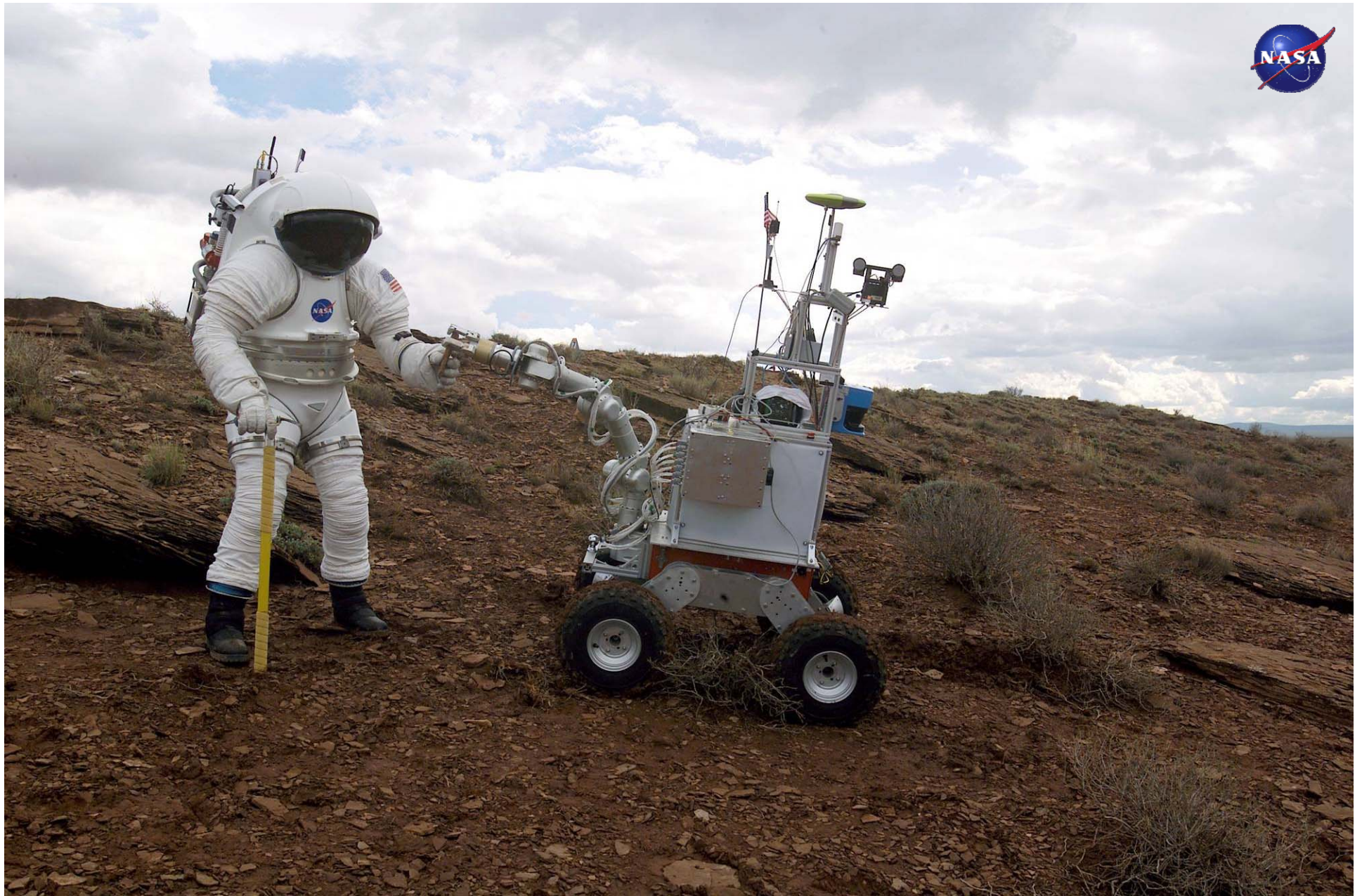
Human/robotic interactive task activities being conducted between MK III suit subject and EVA Robotic Assistant (ERA) vehicle
