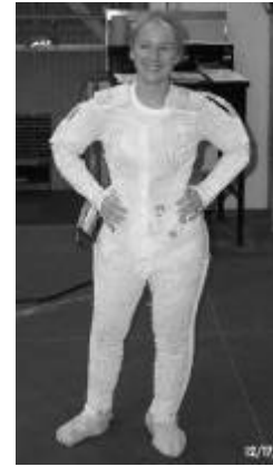
Nylon Spandex/SWNT Fabric for Spacesuits
