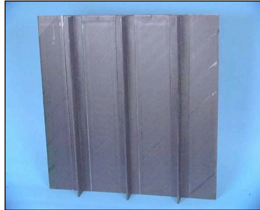
Figure 33 – A [\pm 45^\circ/0^\circ_2/90^\circ/0^\circ_2/\pm 45^\circ] s skin stringer laminate fabricated entirely out-of-the-autoclave using primary bonding. Many IM-7/PEEK, PIXA-M, and PETI-5 panels have been made by this process.
