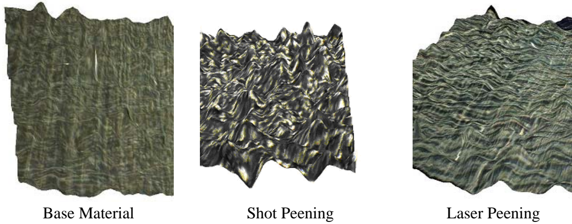
Figure 10: A 3d rendering of the surface roughness resulting from different peening techniques
