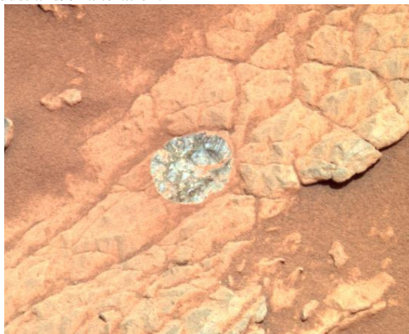
Figure 2. Portion of Pancam false-color image (P2575, Sol 690, L4, L5 and L6 filters) of Algonquin target Iroquet showing RAT brush. Hollows on the outcrop surface caused by cracks still contain dust, which contaminate the post-brush analysis.
