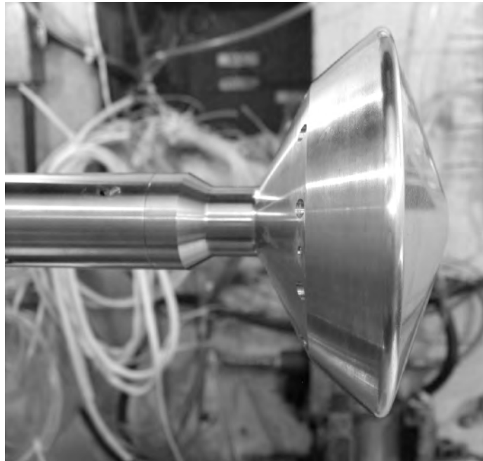
Figure 2. Close-up view of MSL model in NASA LaRC 20-Inch Mach 6 Air Tunnel (retracted into model box)
