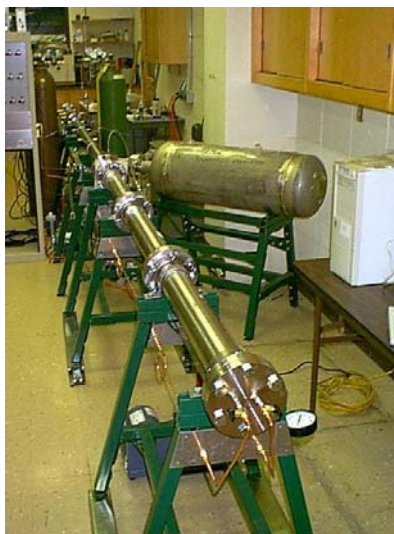
Figure 1: The UDRI high pressure, single pulse, reflected shock tube as viewed from the driver section.
