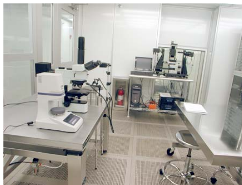
Fig. 3. Air-bearing table, direct thickness measure, bright field/dark field microscope, ellipsometer in ISO Class 4 lab.
