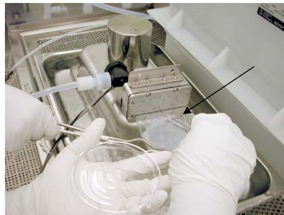
Figure 1: UPW/Megasonic cleaning set-up for small fragments. Fragment (arrow) is gripped with tweezers only on edge and held in flowing stream for 5 minutes.
