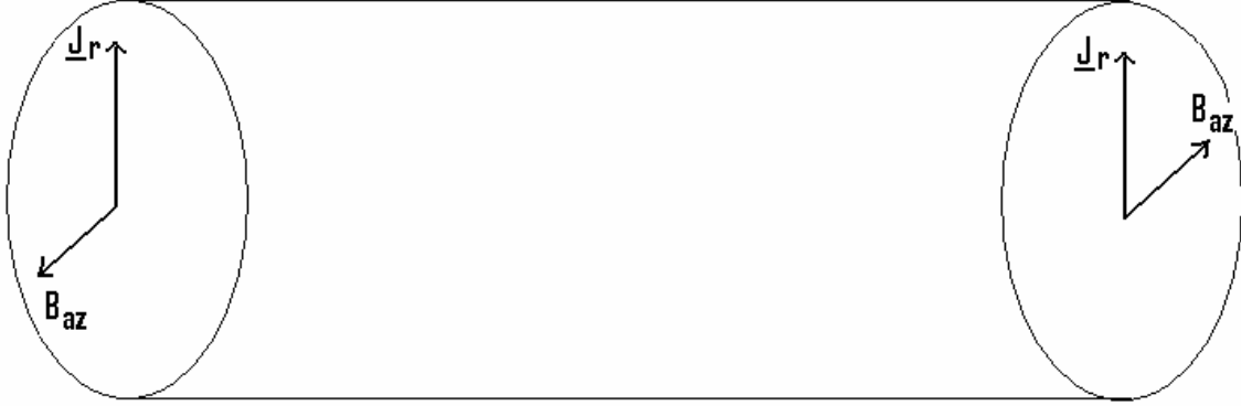
Figure 1. Schematic representation of the double shock generation at the boundaries using radial currents with their accompanying azimuthal magnetic fields.
