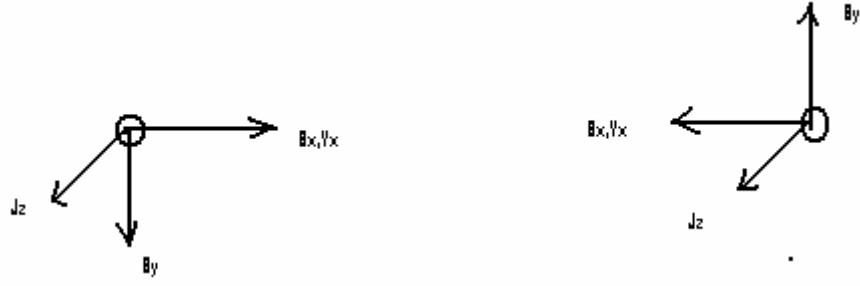
Figure 2. The field and current geometry used in the model. These represent the applied currents and their accompanying fields at the two ends of the proposed device.
