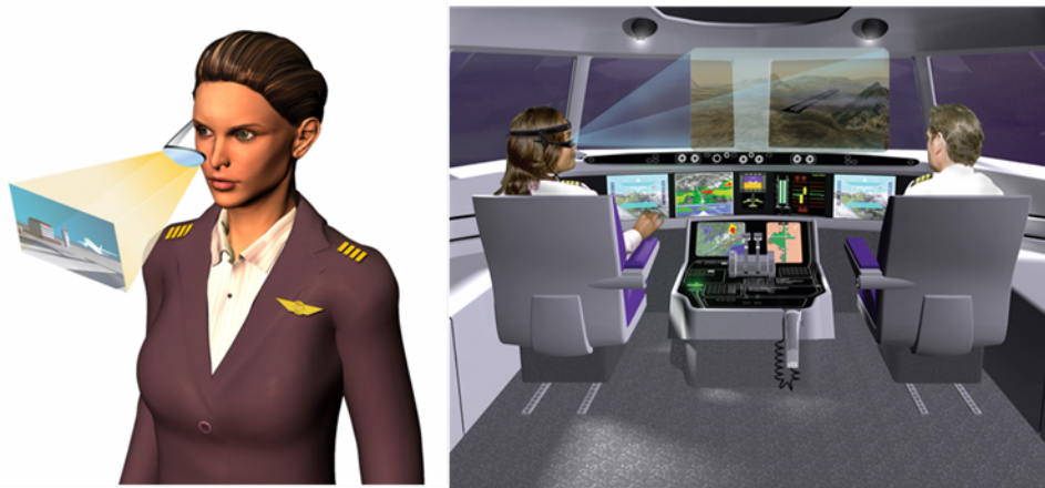
Figure 5. A Synthetic Vision enhanced HWD with a head tracker has unlimited field-of-regard.
