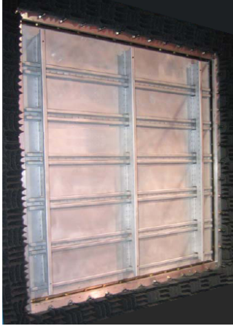
Figure 3: Photograph of the stiffened aluminum test panel.
