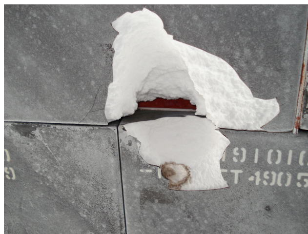
Figure 4. Cavity identified during STS-118.
