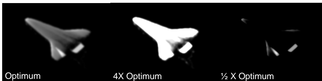
Figure 4. Simulation of variation of exposure setting for a given sensor. Left image shows optimal setting, center image shows a 4 times overexposure and right shows one half underexposure. High temperature laminar flow depicted on right wing in this series of images. Note that turbulent wedge is depicted on left side here. Whiel flight experiment will have it on the right side (as seen from this angle).
