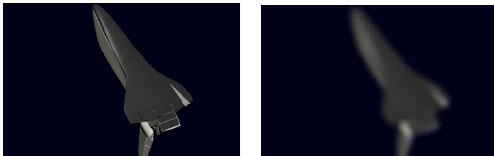
Figure 8. Left image is a “perfect” rendering with no blur, right image has a 10 pixel Gaussian point spread function applied to it.
