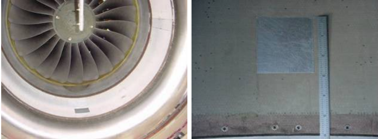
Figure 642. Configuration 47: Square Patch, Away From Fan, At Current Inlet Repair Limits.
