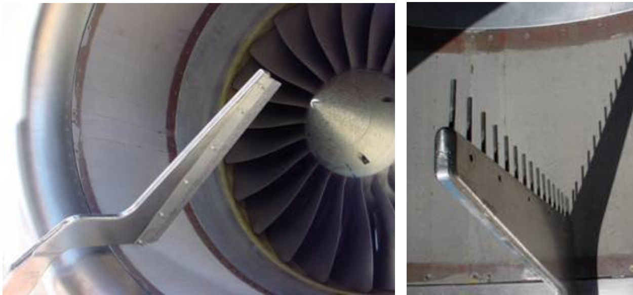
Figure 643. Configuration 39: Fully Treated Inlet With The Rake Transducers Positioned 25 Percent Aft Of The Treated Leading Edge.
