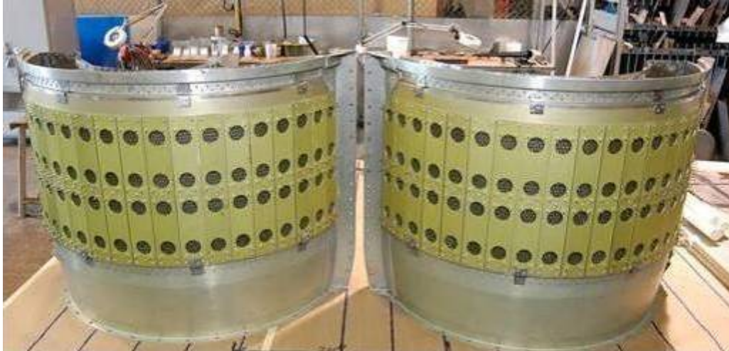
Figure 37. This External View Of The C-Ducts Shows Where The Adaptive HQ-Tubes Are Installed.
