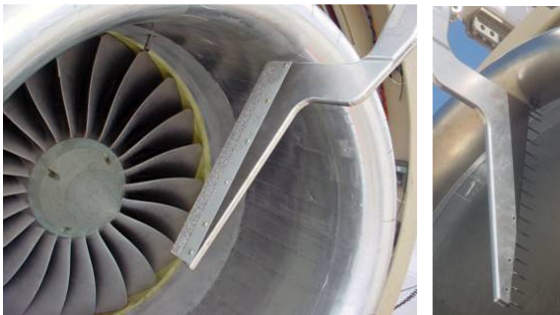
Figure 636. Configurations 38: Fully Hardwall Inlet With The Rake Transducers Positioned At The Throat Location.
