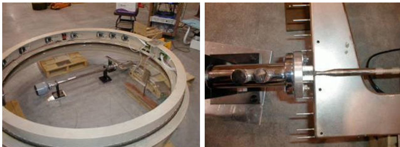
Figure 628. An Impedance Tube Was Used To Excite Two Transducers At A Time To A Sound Pressure Level Established By A Reference Microphone.
