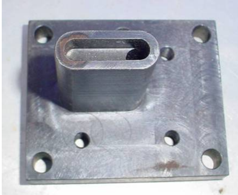
Figure 278. The Hot Film Survey Probe Is Retracted Into A Cavity In The Insert Adapter Pad To Protect It During Installation And Removal.
