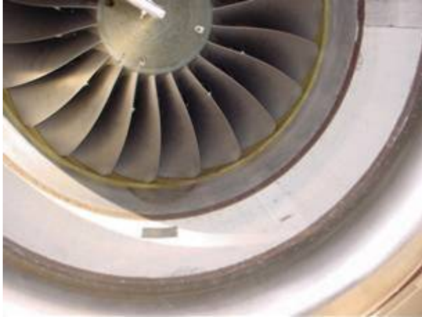
Figure 639. Configuration 44: Square Patch, Close To Fan, At Current Inlet Repair Limits.
