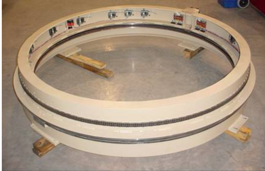
Figure 319. Electrical Installation Of The DC Power Converters, Signal Amplifier Cards, And Wireless Transmitters Into The Rotating Rake Was Completed.
