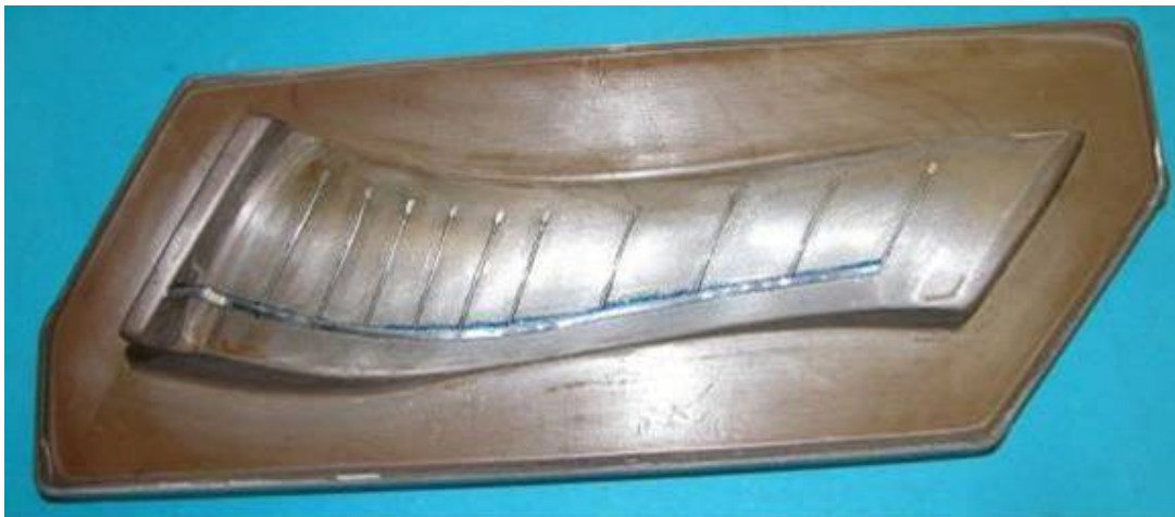
Figure 291. Rectangular Standoffs Were Glued To The Two Halves Of The Vane Mold To Create Recesses In A New Vane.
