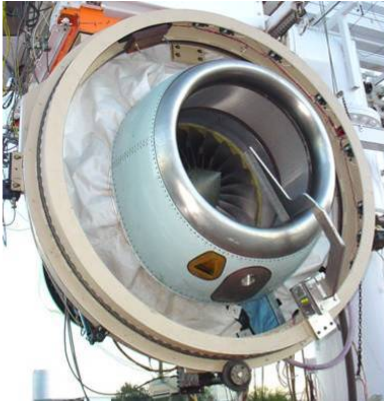
Figure 634. Inlet Rotating Rake Installed On The TECH977 Engine.
