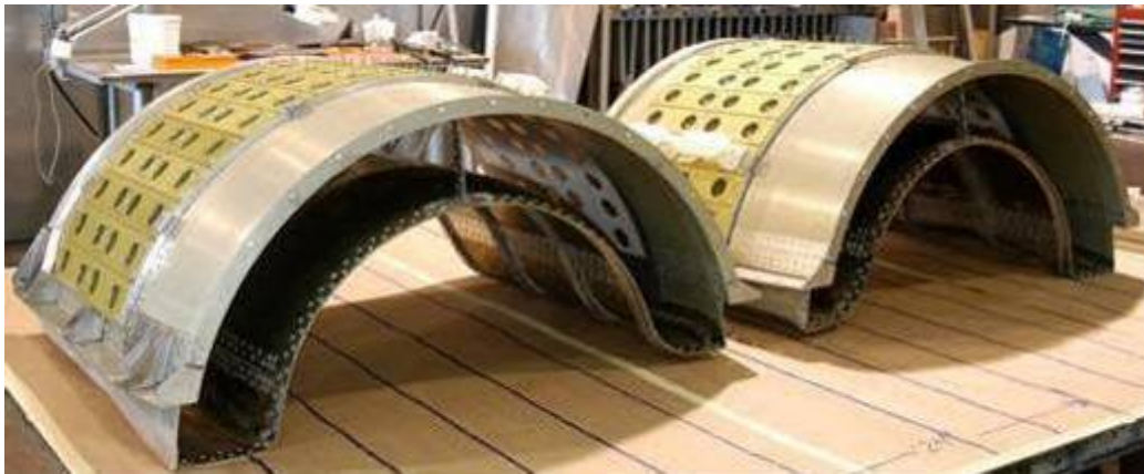
Figure 38. This External View Of The C-Ducts Shows The Flow Path Of The C-Ducts And The Passive Liner With The Cut-Outs For The Sound To Enter The HQ-Tubes.
