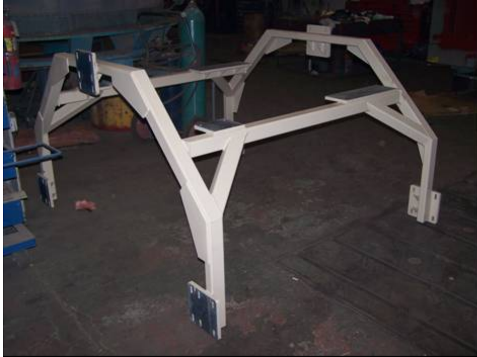
Figure 313. Fabrication Of The Rotating Rake Support Frame Was Completed.
