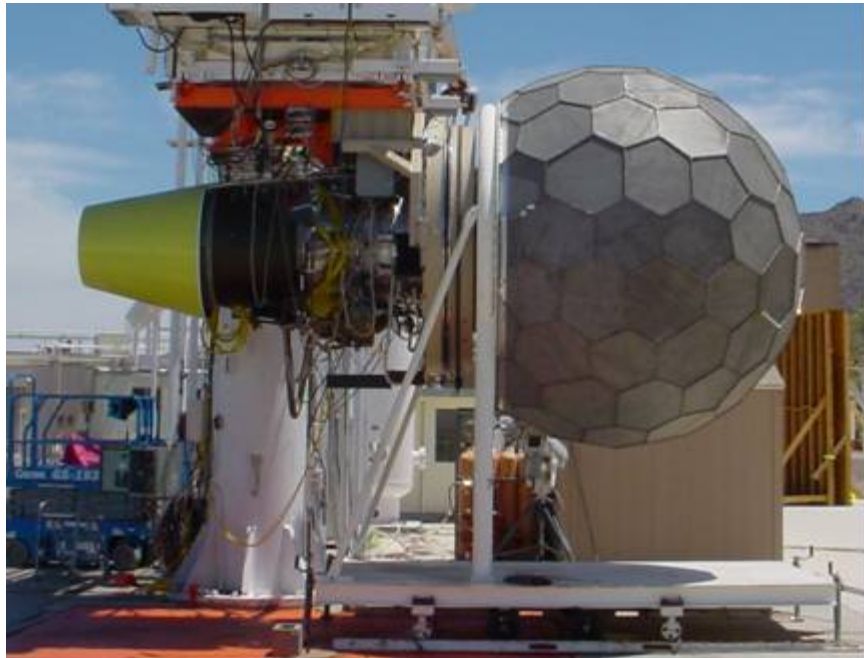
Figure 615. A Preliminary Engine Test Was Conducted Using The Rotating Rake With The Inflow Control Device Installed.
