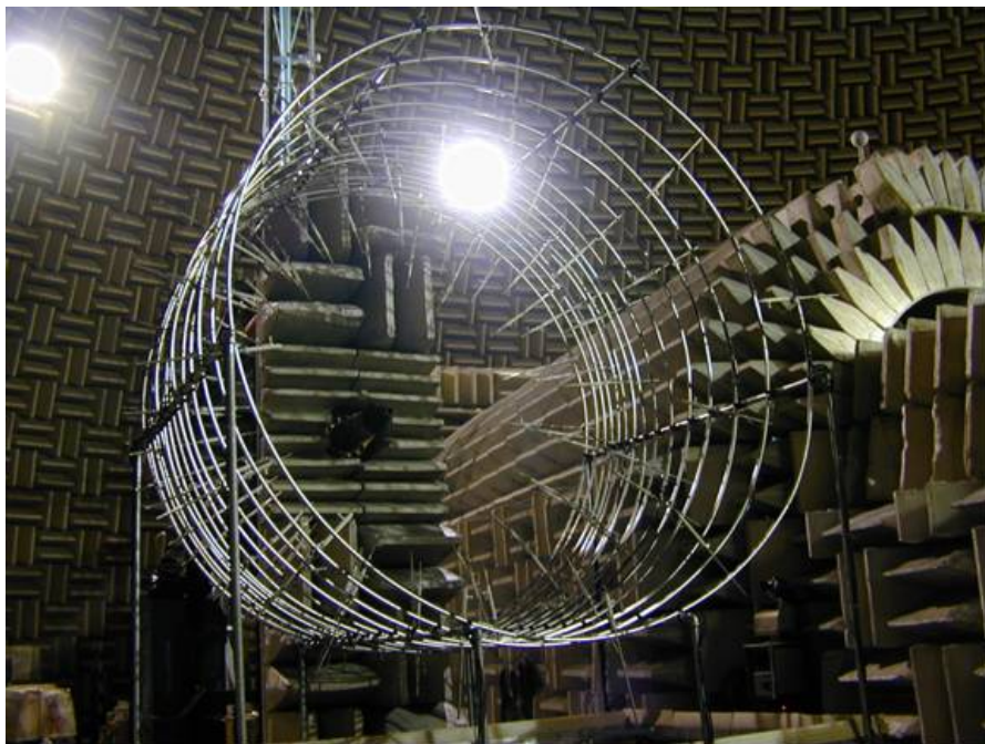
Figure 264. Cage Array Used In The 2003 NASA Glenn Test.
