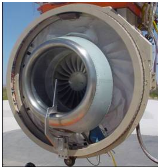
Figure 613. A Sailcloth Was Cannibalized And Used To Prevent Flow Between The Rotating Rake And The Engine.
