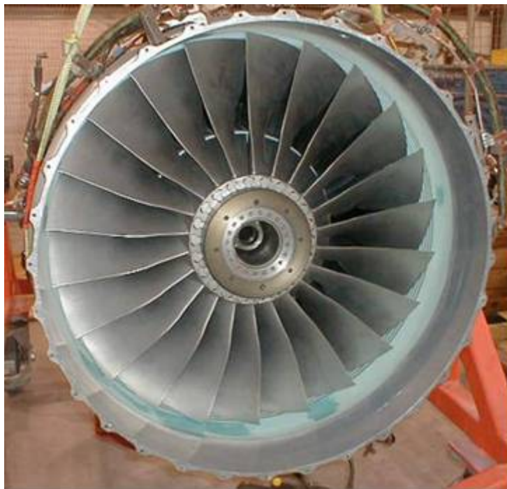
Figure 161. The Engine Scale Quiet High Speed Fan II Has Been Installed On The TECH7000 For A Fit Check.
