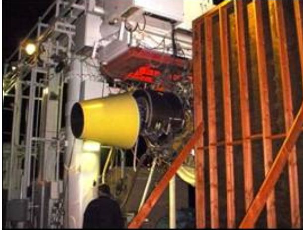
Figure 324. The Photographs Show The Baseline TECH977 Engine Configuration With The Barriers In The Forward Position.
