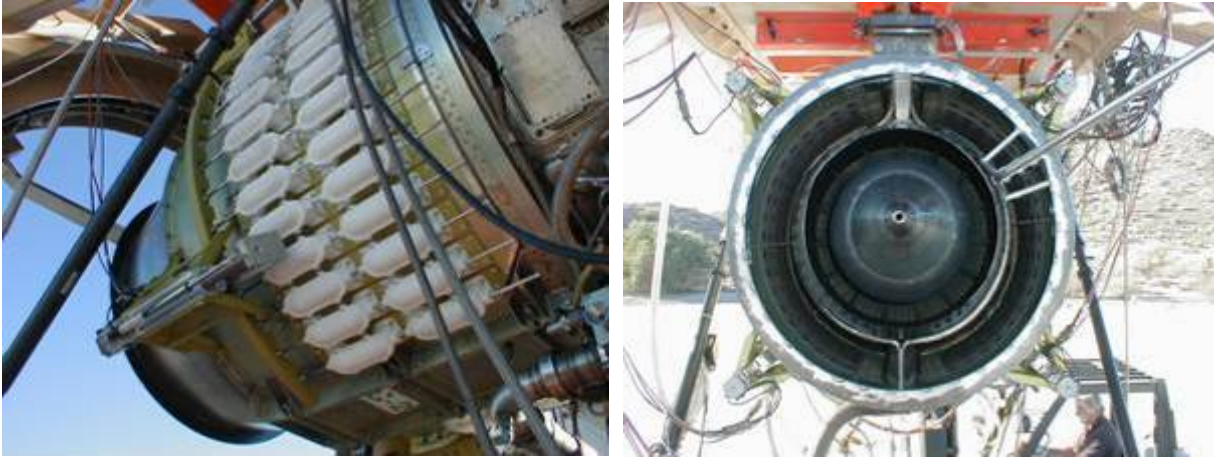
Figure 662. Exhaust Rotating Rake Test Configuration 73, Acoustically Treated Duct With HQ Tube Balls In Forward Position, Was Completed On March 8, 2007.
