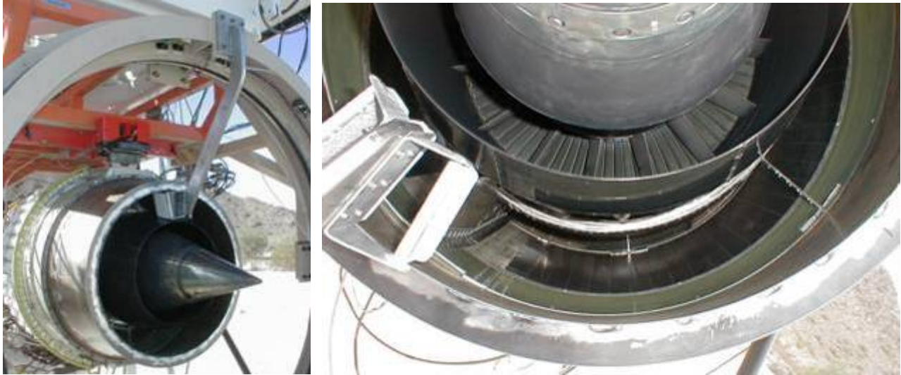
Figure 660. Testing Of Exhaust Rotating Rake Configuration 72 [Left], With The Liner And The HQ Tubes Taped Over [Right], Was Completed On March 6, 2007.
