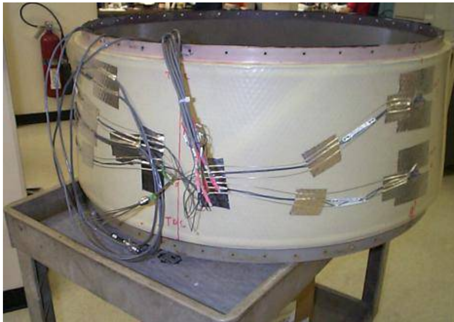
Figure 463. In-Situ Impedance Microphones Were Installed In The Inner Barrel Of A TECH7000 Inlet.
