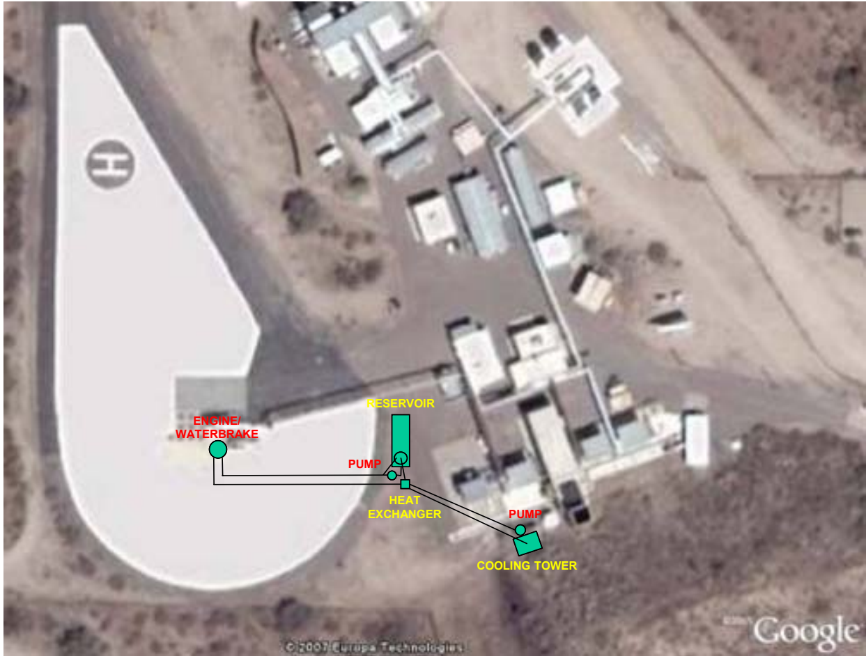
Figure 485. Run Without Fan Water Cooling Layout.
