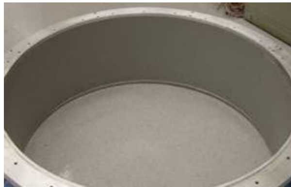
Figure 100. SDOF Linear Liner Used In The ANCF Rig.
