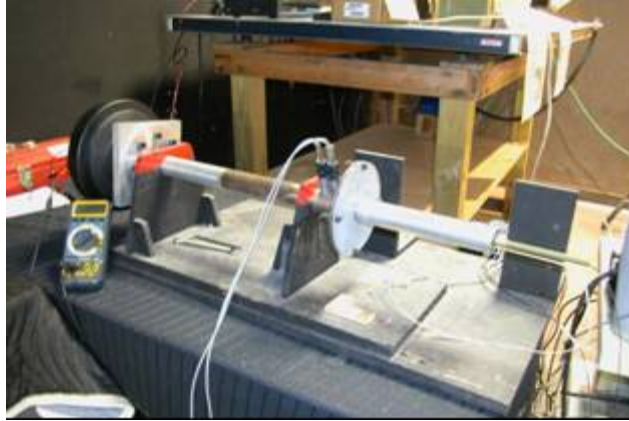
Figure 205. GTRI Normal Incidence Impedance Tube; 1.12-Inch Diameter.
