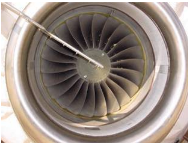
Figure 641. Configuration 46: Square Patch, Close To Fan, At Twice Current Inlet Repair Limits.
