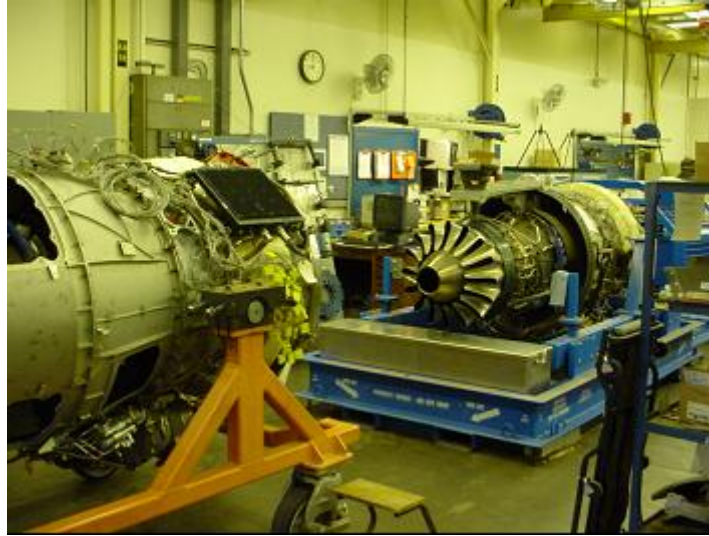
Figure 159. The Engine On The Left Is The TECH7000 And The Engine To The Right Is The TECH977.
