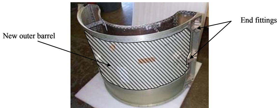
Figure 4. A Photograph Of The Existing TECH977 C-Duct Shows The Zone Where The HQ-Tubes Will Be Installed.
