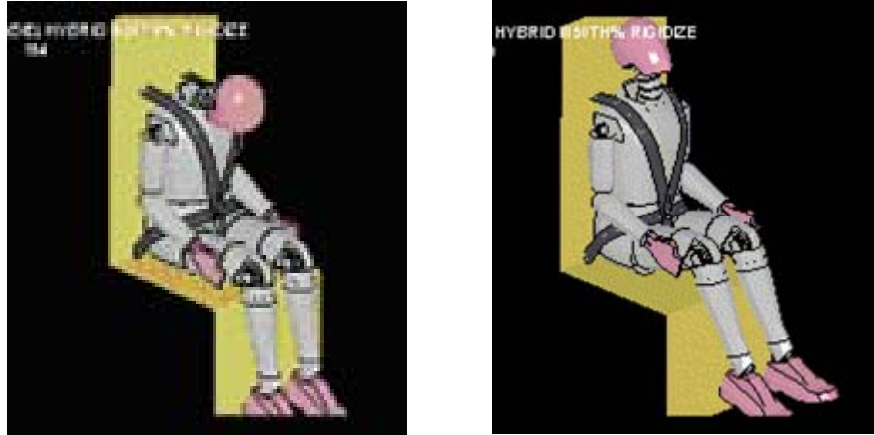
Figure 6.—Hybrid III crash test dummy response at intermediate time steps.
