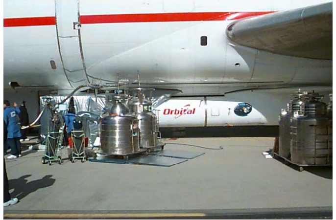
Figure 5.—Pegasus attached to L-1011 Aircraft. Note the band around the fuselage containing the hydrogen vent. The helium dewars in the pictures are for maintaining the hydrogen as a solid prior to launch.
