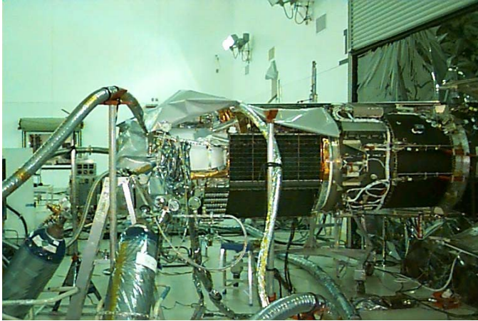
Figure 3.—WIRE in the payload processing facility at WTR at Lompoc, California. This facility is set up to safely handle hydrogen.
