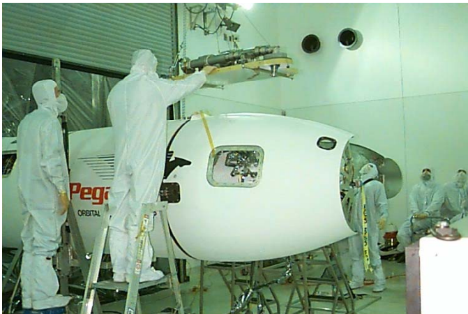
Figure 4.—WIRE mounted into the Pegasus fairing. Note the fairing door used to service the experiment on the “hot pad.”
