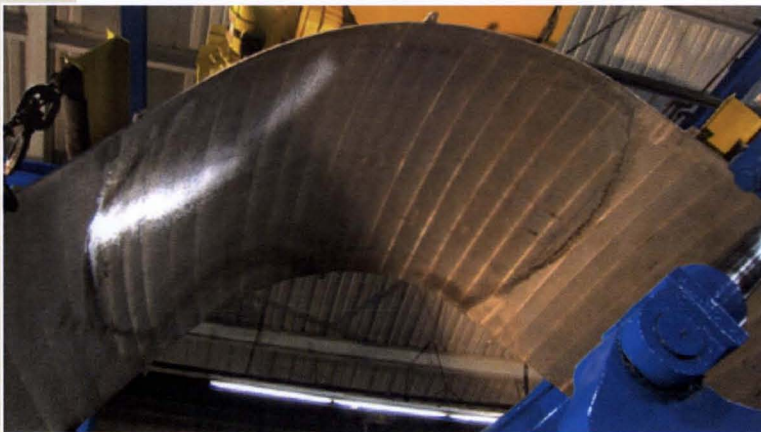
Fabricating Gore Dome Panels for Upper Stage
