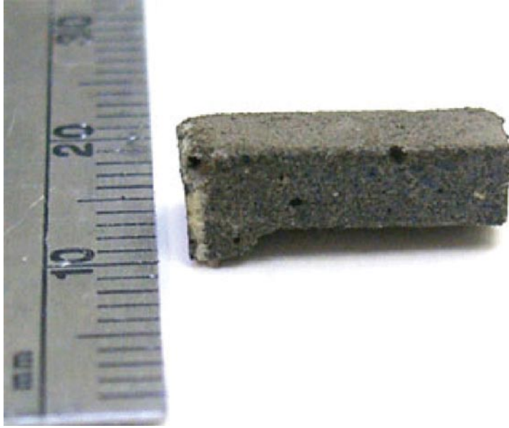
Figure 22. Macrograph of the sulfur - 65 wt. % JSC-1 sample after 8 days in vacuum that represents the green diamond datum point, figure 21. The ‘leg’ inadvertently left on the sample effectively exposed more surface area and resulted in a greater mass of lost sulfur.
