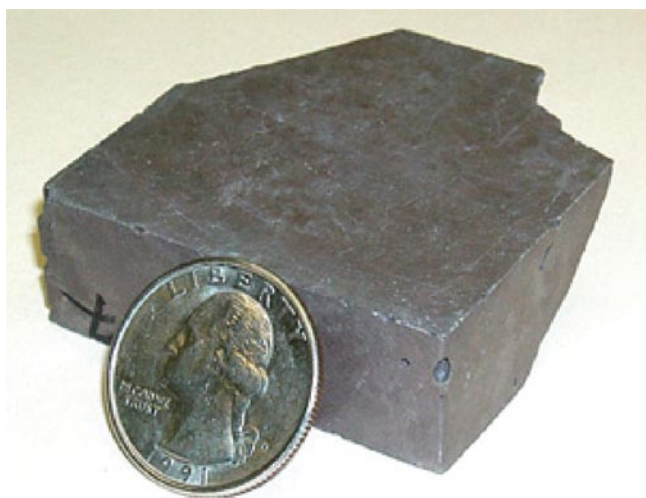
Figure 6. A piece of sulfur-based concrete made at The University of Alabama in Huntsville. The corners were broken off for testing purposes.
