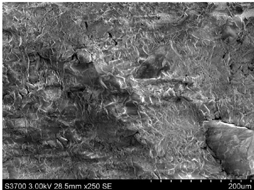
Figure 38. SEM micrograph of a fracture surface from noncycled sample 6 with the same composition as in figure 37, but tested at -101\text{ }^{\circ}\text{C} ( -150\text{ }^{\circ}\text{F} ).
