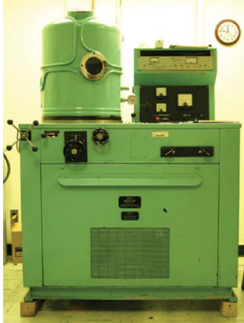
Figure 7. Photograph of the vacuum chamber used for the sublimation experiments.
