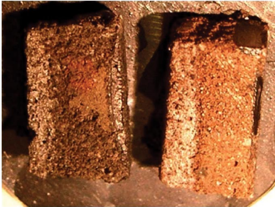
Figure 25. Photograph of two samples exposed to vacuum for 60 days: left: sulfur - 35 wt. % JSC-1 and right: 25% sulfur and 20% silica by weight with 55 wt. % JSC-1.
