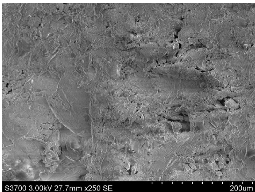
Figure 37. SEM micrograph of a fracture surface from noncycled sample 4, a sulfur with 65 wt. % JSC-1 sample tested at 21\text{ }^{\circ}\text{C} ( 70\text{ }^{\circ}\text{F} ).
