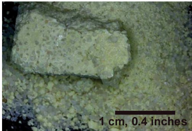
Figure 42. Photograph of a sample like that seen in figure 7 which was cycled 20 times between room temperature and -196\text{ }^{\circ}\text{C} ( -321\text{ }^{\circ}\text{F} ). Crumbling of the sample with free grains of silica is seen.
