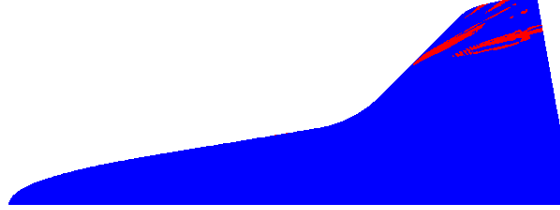
Figure 5. Absolute values of percentage extrapolation errors for Re_k boundary layer transition parameter (23). Red is more than 4.5%. Blue is less than 4.5%.
