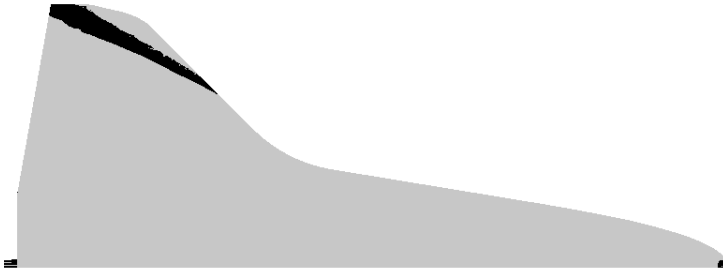
Figure 8. Absolute values of percentage errors for post normal-shock stagnation pressure coefficients. Black is more than 3%.
