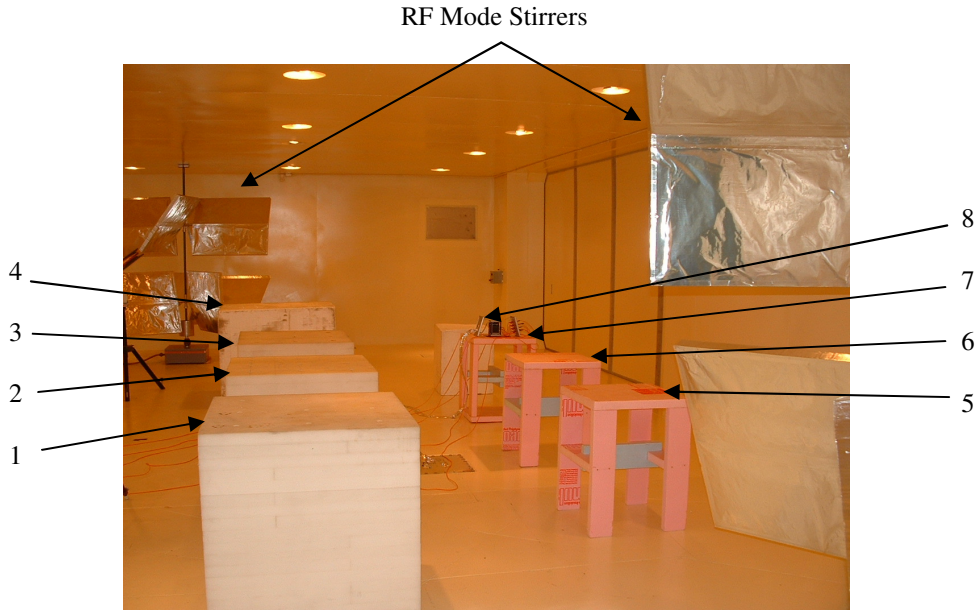
Figure 8: Device Positions inside the Test Chamber
