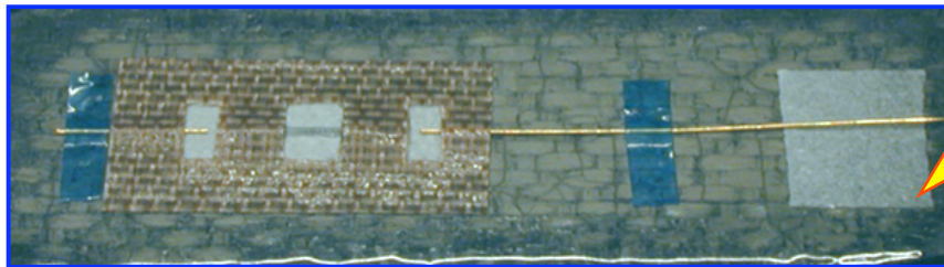
Flame-spray sensor attachment
