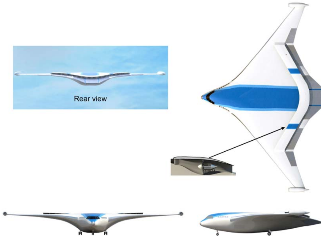
Figure 2.—A notional distributed turboelectric propulsion CESTOL vehicle concept using 16 distributed electric fans driven by superconducting motors with power provided by two wing-tip-mounted turboelectric generators.
