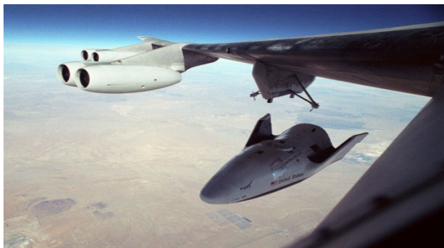
Figure 7.—The X-38 drops from the B52 pylon.
