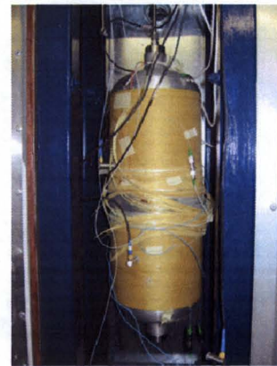
Figure 9 – failed vessel 6.3 inch COPV
