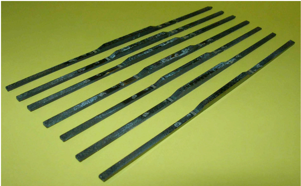
(b). Specimen 10B-03 cut into seven slices.
