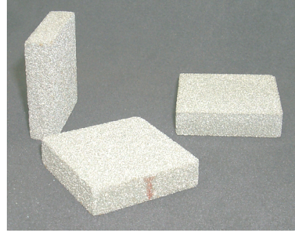
Figure 2. Photograph of Foam-metal Samples (2" x 2" x 0.425")
