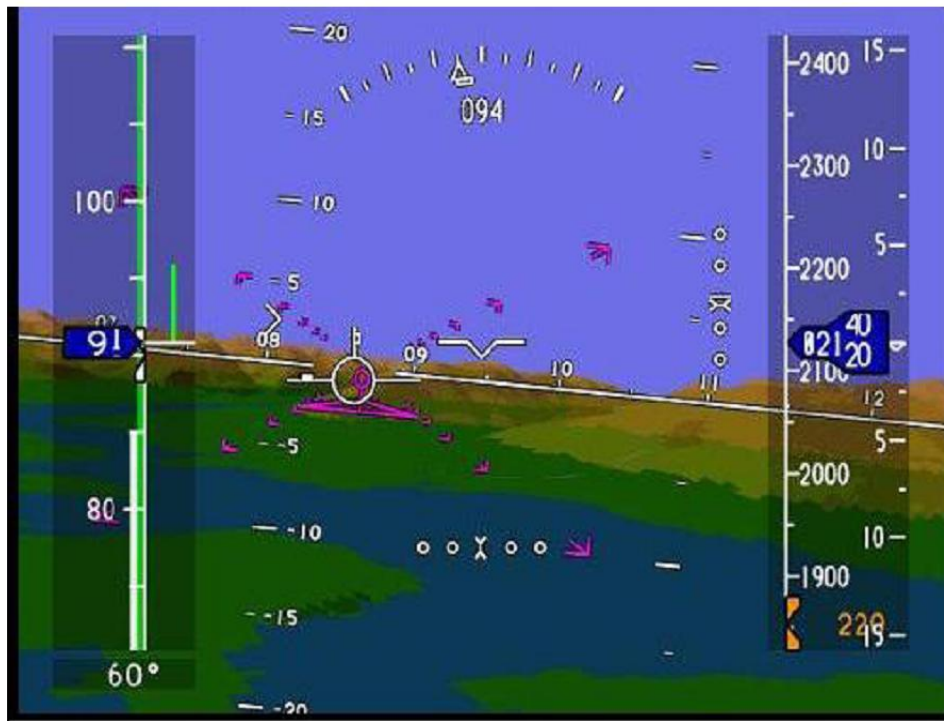
Figure 78. GA Crow's Foot Tunnel with Ghost Aircraft display concept.
