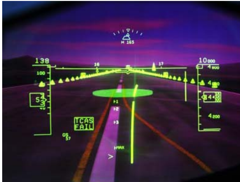
Figure 14. Illustration of RIPS HUD landing/rollout deceleration guidance format (all HUD symbology is monochrome green).
