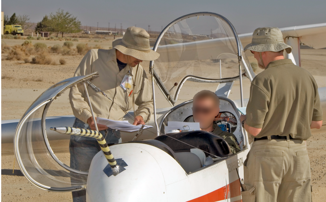
Figure 6. The sailplane’s noseboom-mounted microphone and bullet-nosed windscreen.
