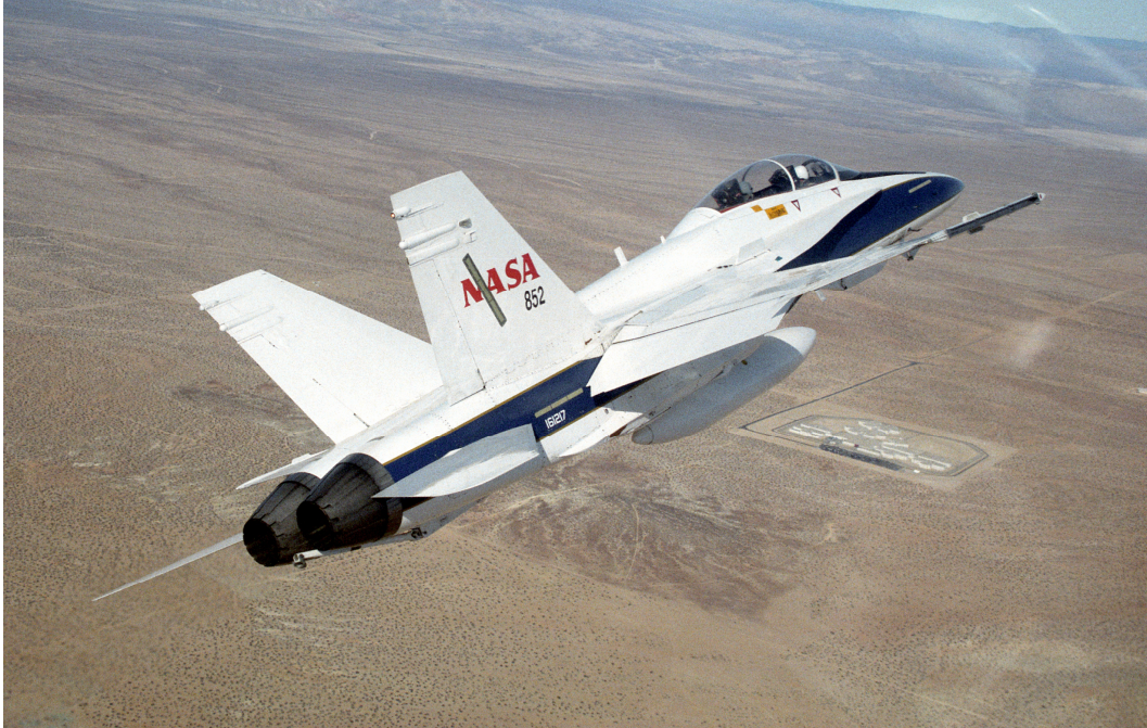
Figure 1. The instrumented NASA F-18B airplane, tail number 852, used for most of the sonic boom flights.
