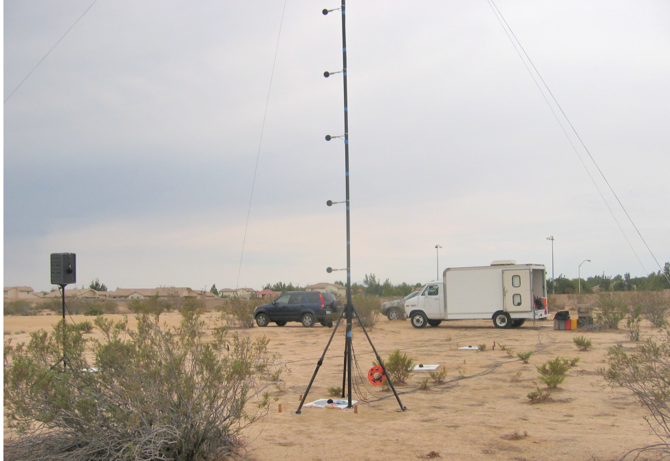
Figure 4. Tower, 5 m south and 5 m east groundboards, 10 m south groundboard, white noise loudspeaker, and support vehicles.
