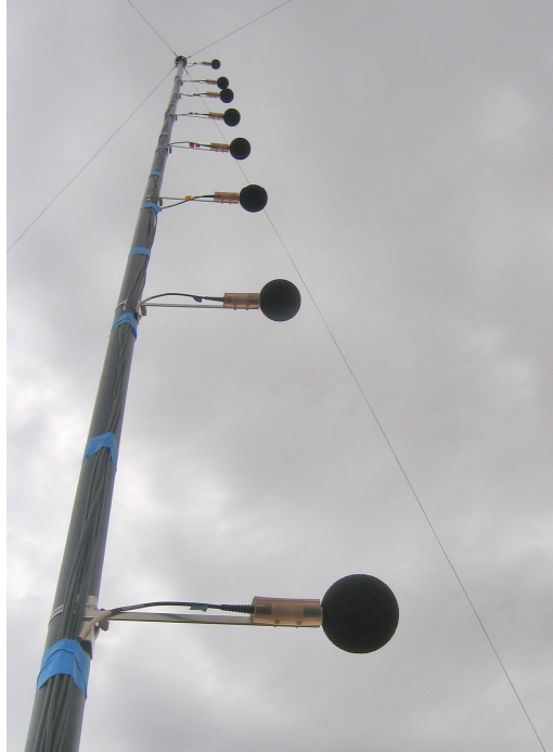
Figure 2. The 10 m tall tower with microphones at 2 m to 10 m; the four guy-wires can be seen connected at the apex of the tower.
