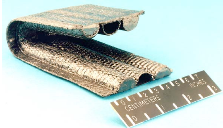
Figure 39. Photograph of Mo-Re tube embedded in C/C illustrating the design of a NASP heat-pipe-cooled wing leading edge.
