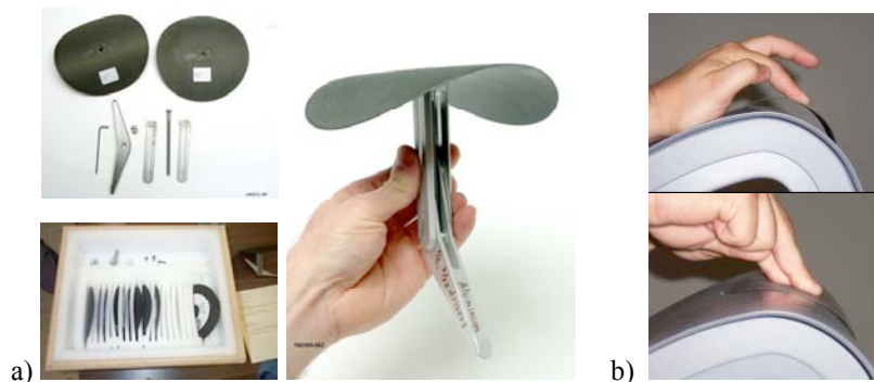
Figure 36. Photograph of Space Shuttle Orbiter wing leading edge plug repair a) C/SiC cover plates and TZM attachment mechanism, and b) C/SiC cover plate formed around simulated leading edge.
