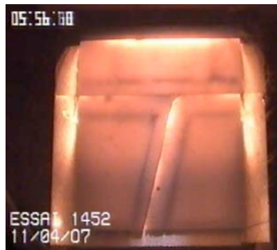
Figure 52. Snecma Propulsion Solide CMC TPS array during arc-jet testing.
