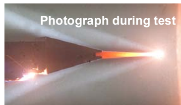
Figure 34. Arc-jet coating evaluation of X-43 leading edges.
