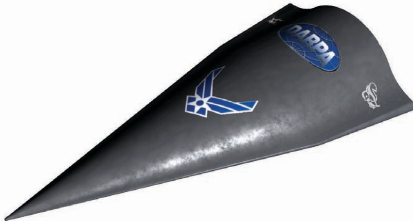
Figure 56. DARPA/Air Force Falcon HTV-2 vehicle, which utilizes a C/C aeroshell.
