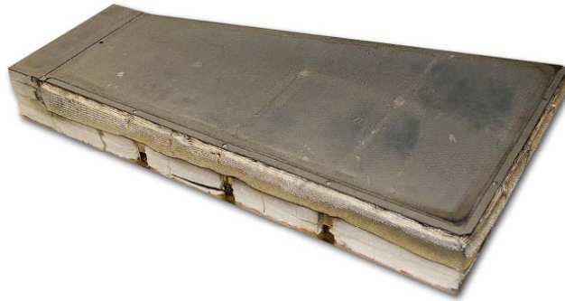
Figure 51. SPS CMC TPS array for mechanical, dynamic, thermal, and thermal-mechanical testing.
