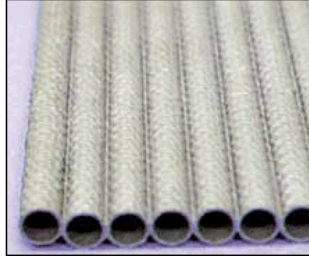
Figure 44. Photograph of an all composite actively cooled test article.
