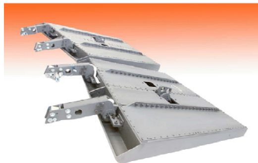
Figure 63. Photograph of the X-38 C/SiC body flaps fabricated by MT Aerospace [30].
