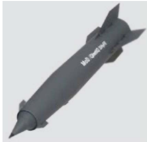
Figure 57. C/SiC load bearing aeroshell utilized on the SHyFE [24].
