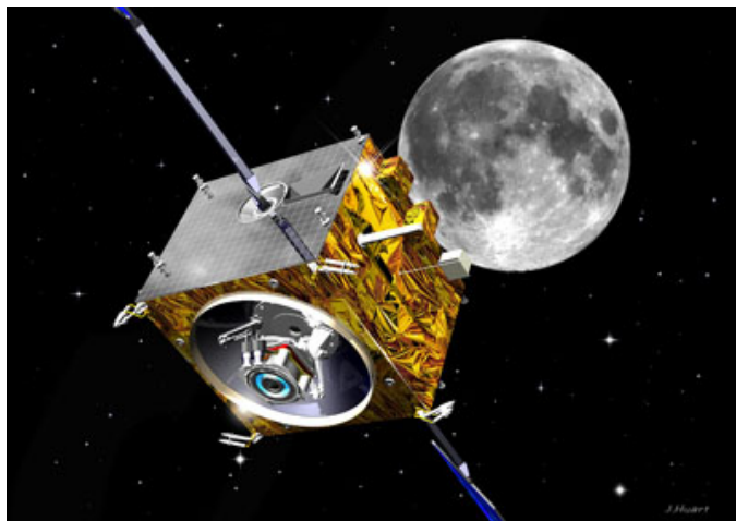
Figure 2.—The European Space Agency's Small Missions for Advanced Research in Technology 1 (SMART-1) Lunar probe.
