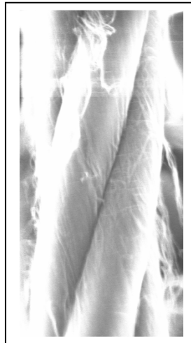
Figure 1. SEM micrograph of a longitudinal view of typical four-ply multi-wall carbon nanotube yarn (2500x; 15kV).
