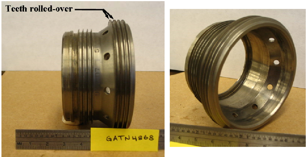
Figure 3.—No. 3 labyrinth seal.
