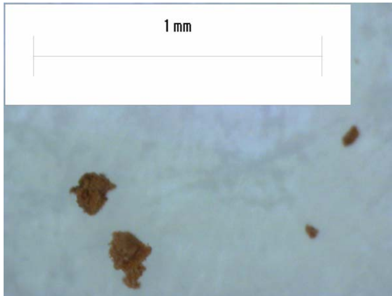
Figure 9.—Close-up micrograph of sand particles from modified CDP seal in figure 5.
