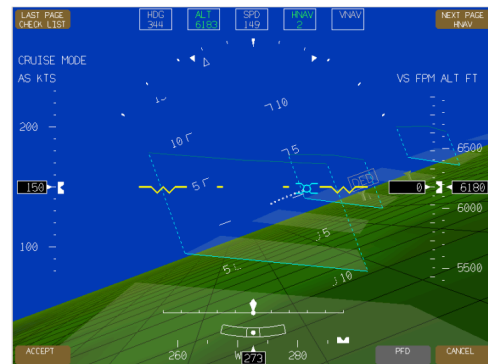
Figure 14. SmartDeck advanced display with SVS/HITS/FD guidance.
