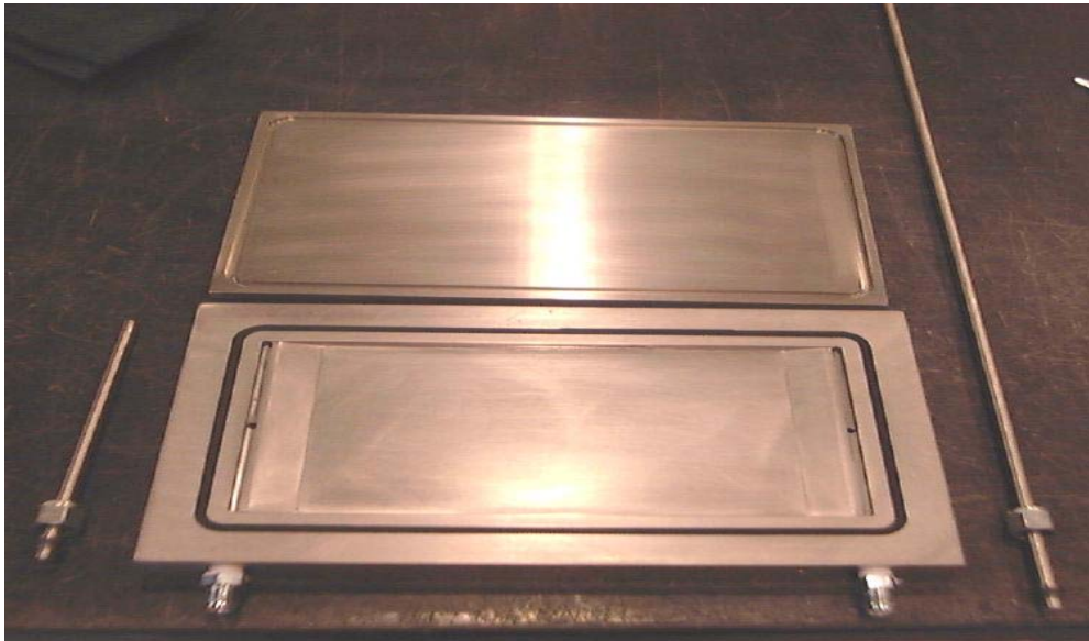
Figure 4: Tool for injection molding of PETI-330/MWNT plaques; a) schematic (all dimensions in cm) b) photograph
