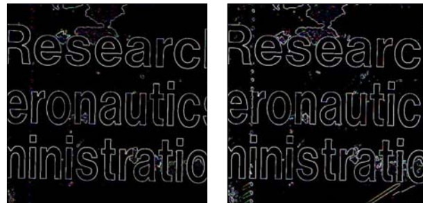
Figure 16. Edge patterns showing small, strong shadows on a scene dominated by reflectance rather than by topography.
