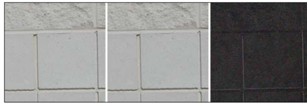
Figure 15. Edge pattern subtraction from correlation limit test. Original images shown to illustrate near-identical scenes.
