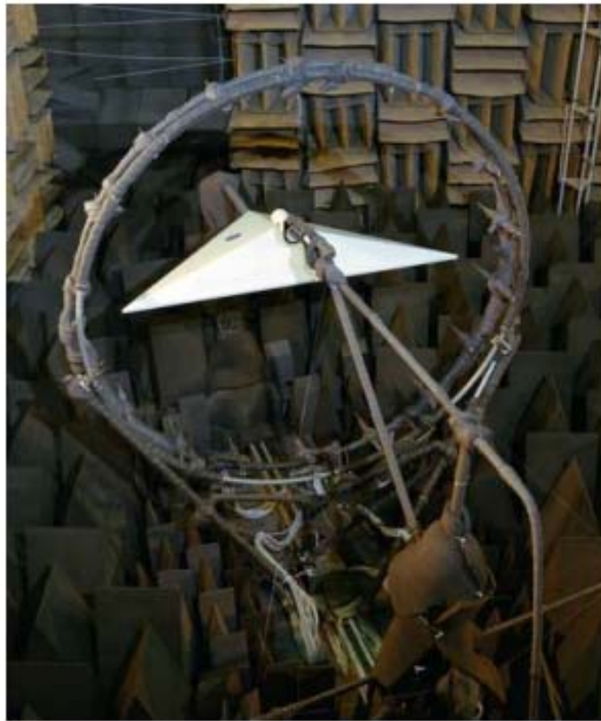
Figure 1. Photograph of wedge-shape airfoil model experiment set-up in anechoic chamber, view looking upstream
