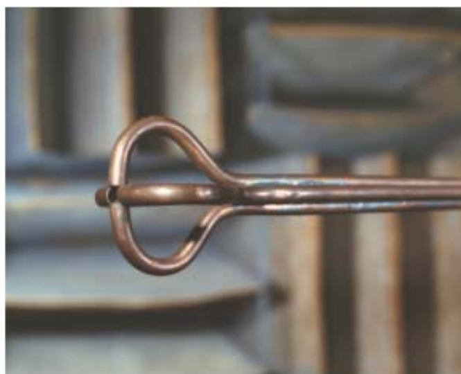
Figure 6. Broadband, high intensity point noise source consisting of four impinging air jets.
