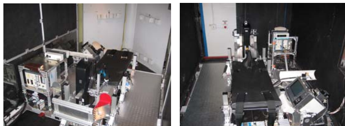
Figures: Subject bed/seat configuration on centrifuge with instrumentation racks.
