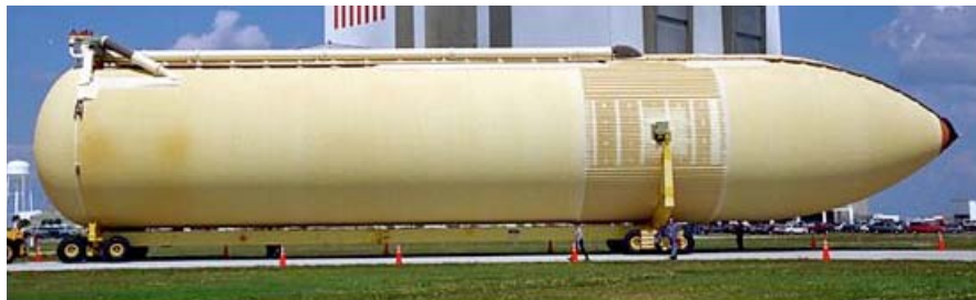
Figure 2. Insulating foam on Space Shuttle External Tank.
