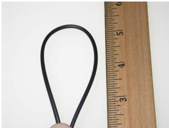
Figure 8(a): No kinks – 30 wt % MWCNT
