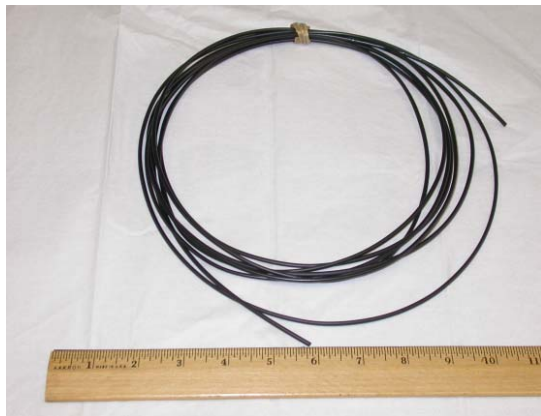
Figure 4: Extruded tubes of Elvax™ 260/MWCNTs
