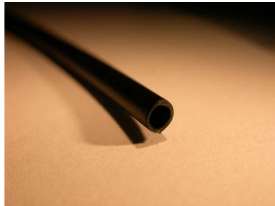
Figure 4: Extruded tubes of Elvax™ 260/MWCNTs
