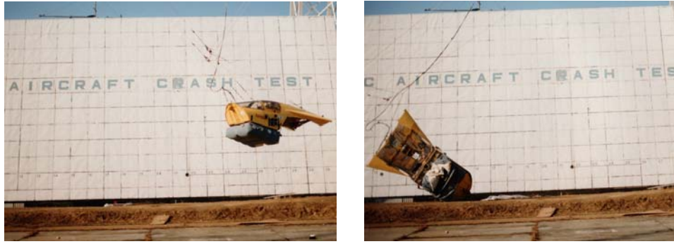
Figure 3. Photographs of an impact test of the F-111 crew escape module with airbag attenuation system.
