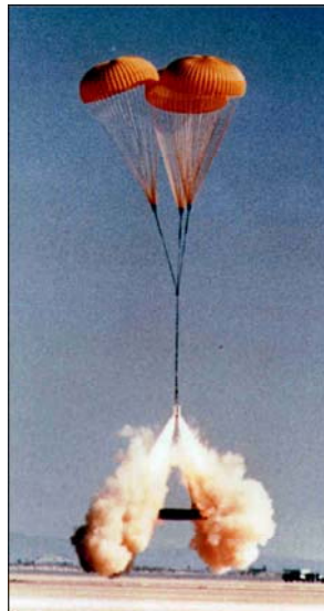
Figure 6. Confluence retrorocket system showing rocket blast just before impact.
