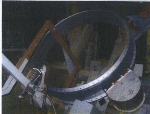
Nozzle Components – Throat Housing
